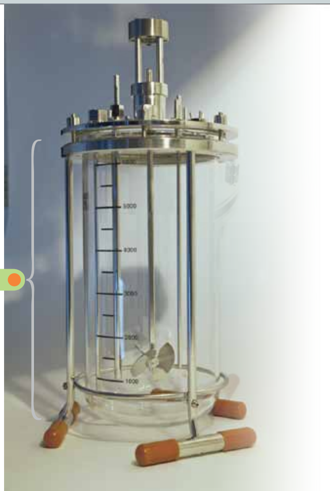
EXAMPLE: 7 L vessel uses 325 mm long sensor
