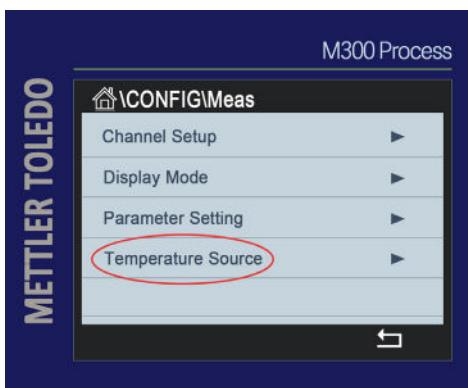
3. Set Sensor to **Fixed** and temperature to 25.000 degrees C.
