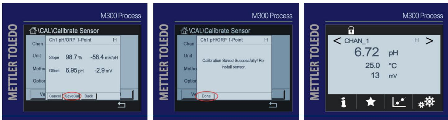
14. The sensor is now ready to be used by transferring the sensor position from Calibration to Measure.
