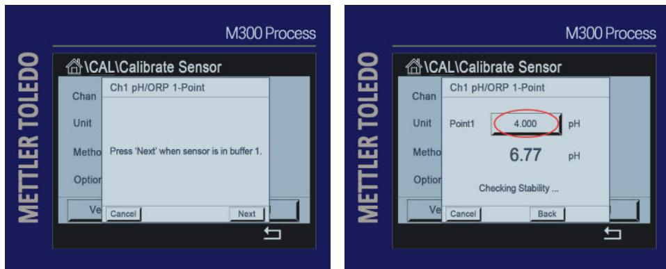
12. Add the 1-pt pH value, and wait enough time to ensure the sensor is thermally equilibrated with the process (up to one hour). Press **OK**.
