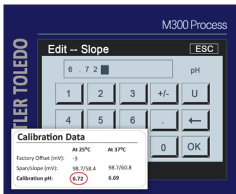
13. The calibration will now be completed and the calibration values will be displayed. Select **SaveCal** to save the calibration data. A message with pop-up that calibration saved successfully. Press **Done**. Finally, go back to Home screen and make sure the pH reading is correct according to the calibration value.
